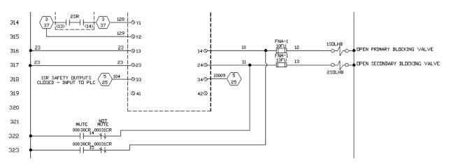
00030CR and 00031CR contacts mute the two-hand control safety relay contacts, keeping power to the hydraulic blocking valves. The mute timing is controlled by the PLC at those times in the cycle when it is safe for the operator to release the two-hand control. The *Not Mute* provides the redundancy as required in Control Reliable circuits and single point-of-failure protection as described in the *Failure Mode Considerations* section of this document.
