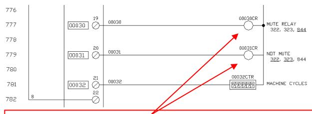
00030CR and 00031CR are direct-drive relays with positively guided contacts. They can be controlled by any PLC output card that does not control hazardous motions. 00030CR is identified as the *Mute Relay* which energizes to provide power to the safety blocking valves when it is safe to release the two-hand control. 00031CR is the NOT state of the 00030CR
