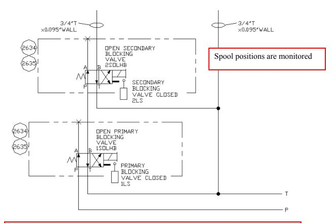
Hydraulic fluid power to all motion valves was initially removed via redundant blocking valves, whenever the two-hand control was released.
