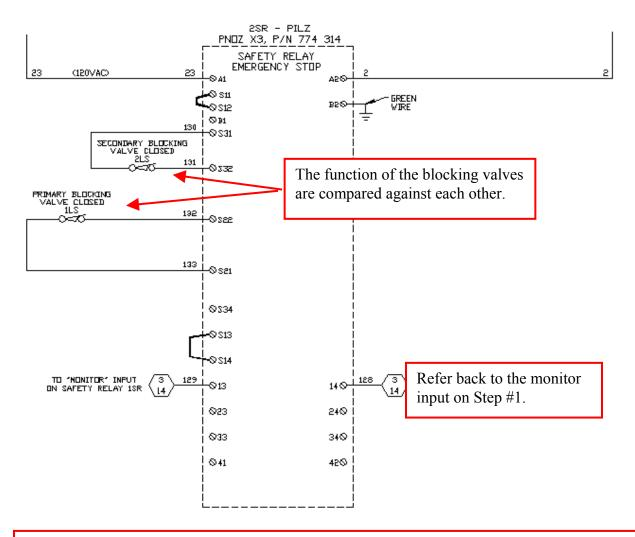
The final switching devices, in this case the redundant hydraulic blocking valves, are monitored. When 1SR kills power to the blocking valves, both inputs to 2SR must close, indicating that both blocking valves have functioned, in order for 2SR's output to pass power to the *Monitor* input of 1SR. This allows 1SR to reset the next time the two-hand inputs are pressed.
